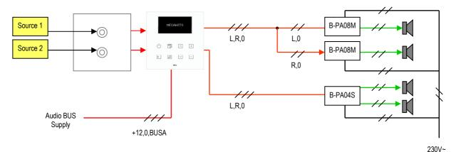
The audio unit receives the 12V power from the D-PS12V15W installed in the switchboard and the audio BUS that comes from the feeder D-BUSAUDIO.
