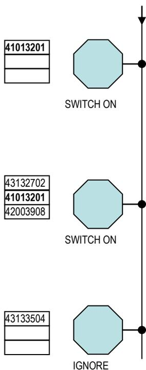
The last one is a command that does not have any electrical function but it only serves to receive command buttons. It is installed for instance in a hallway where we need several command points for the same light. In this case one of the commands executes the function and the other just support the buttons.
