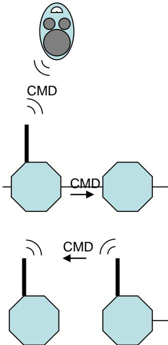
The ONLY system was designed in a way to allow communication both by BUS line and by radio frequency or other wireless system.
