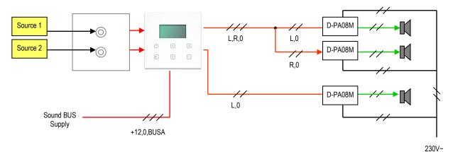
The sound unit receives the 12V power from the D-PS12V15W installed in the switchboard and the audio BUS that comes from the feeder D-BUSAUDIO.
