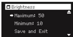
To adjust the brightness level of the OLED, press key
