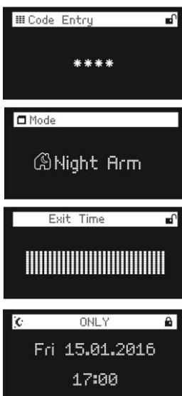
The night mode allows protection of the house, arming only the peripheral and partial zones, allowing the circulation inside the house.
