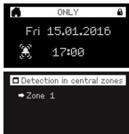
On the keyboard, in case of an alarm, the icon is shown on the display, simultaneously the internal beeper of the keypad sounds.
